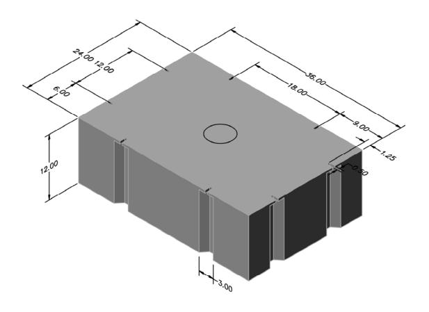
D335 24"x36"x12" 335 lbs of lift capacity 8 attachments on 12" and 18" ctrs.
